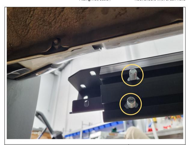
50. Slide in 2x M10x25 hex bolts into the front open end of the extrusion as shown.
