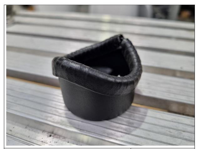
66. Fit supplied pinch weld around the curved edge of the spigot. Trim with side cutters if oversized.
