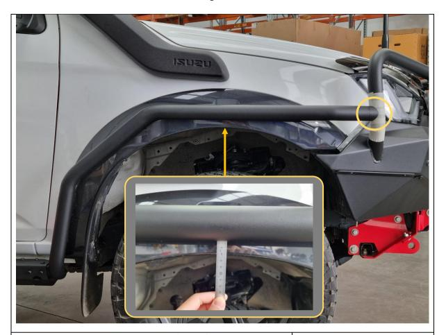
54. Place the spigot end assembly (circled) in between the scrub rail and Toro bar.
