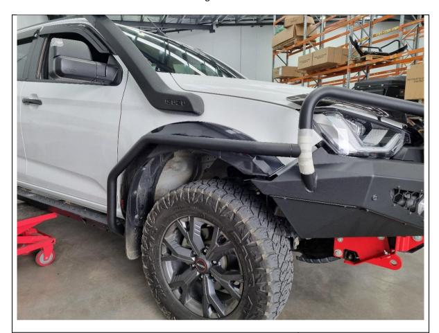
51. Perform a dry test fit of the scrub rail by sliding it into the open end of the slider step.
